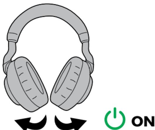
The headphones automatically power on when the earcups are rotated into the wearing position.
