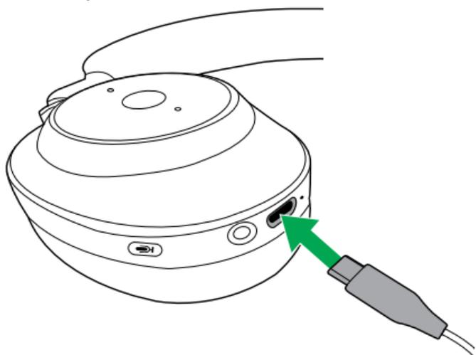
It takes approx. 2.5 hours to fully charge the battery. If the headset is fully out of battery, 15 minutes of charging will give 5 hours of battery.
